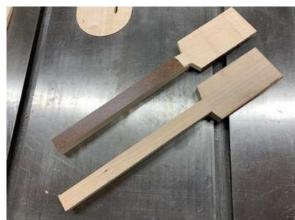
Lay out a tapered paddle that is about 3/8 inch wide where it meets the handle, and bandsaw that out. You don't have to saw out the tapered section at first; you can save it for the end, or keep it thick for more secure work holding while turning, or for alternate utensil shapes.
