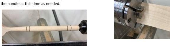
Remove the item from the lathe, and sand the paddle end to remove the bandsaw marks and bring it to a workable thickness at the end, with a smooth transition to the handle. Sand the corners of the paddle to a smooth radius, one larger than the other. Finish sanding for smoothness, rounding all sharp corners and removing any tool marks.
