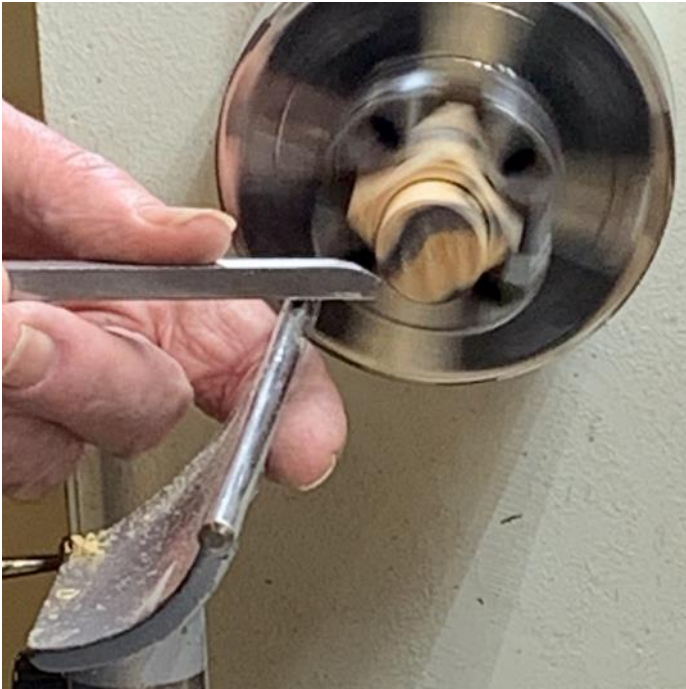
These two pictures show the position of the male chaser and the formation of the threads
